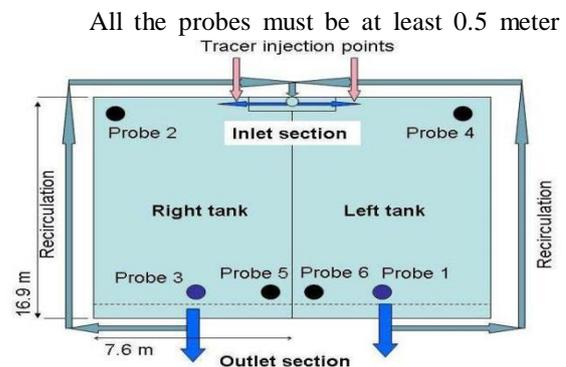
from any wall of the tanks just to avoid mechanical shocks that could damage the detector.
