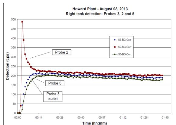
Fig. 6. Radiotracer detection in the right tank
